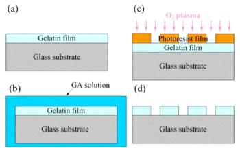
Figure 1. The patterning process of GA-crosslinked gelatin: (a) Spin-coating pure gelatin film at 50 °C, drying for 1 day; (b) Crosslinking gelatin film in 50% GA solution; (c) Patterning a positive-toned photoresist mask on the gelatin film and etching by  $O_2$  plasma; (d) Stripping photoresist by acetone.
