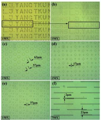
Figure 2. The fabricated gelatin micropatterns: (a) before stripping the photoresist mask; (b) stripping the photoresist, micro letter pattern of 17  $\mu$ m width; (c) micro honeycomb patterns; (d) micro "cross" patterns, the largest width is 17  $\mu$ m; (e) micro square patterns, the largest width is 37  $\mu$ m; (f) microstrips lines with 2  $\mu$ m width, 90  $\mu$ m length and the gap between two lines is 23  $\mu$ m.
