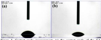
Figure 4. Contact angle measurement: (a) the contact angle of the GAcrosslinked gelatin film; (b) the contact angle on the glass substrate.
