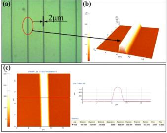
Figure 3. Thickness measurement of gelatin micropattern scanned by AFM: (a) the scanned sample of microstrips lines with 2  $\mu$ m width; (b) AFM scanning picture of microstrip gelatin; (c) the cross-section line profile of microstrips lines with 0.8  $\mu$ m thickness.
